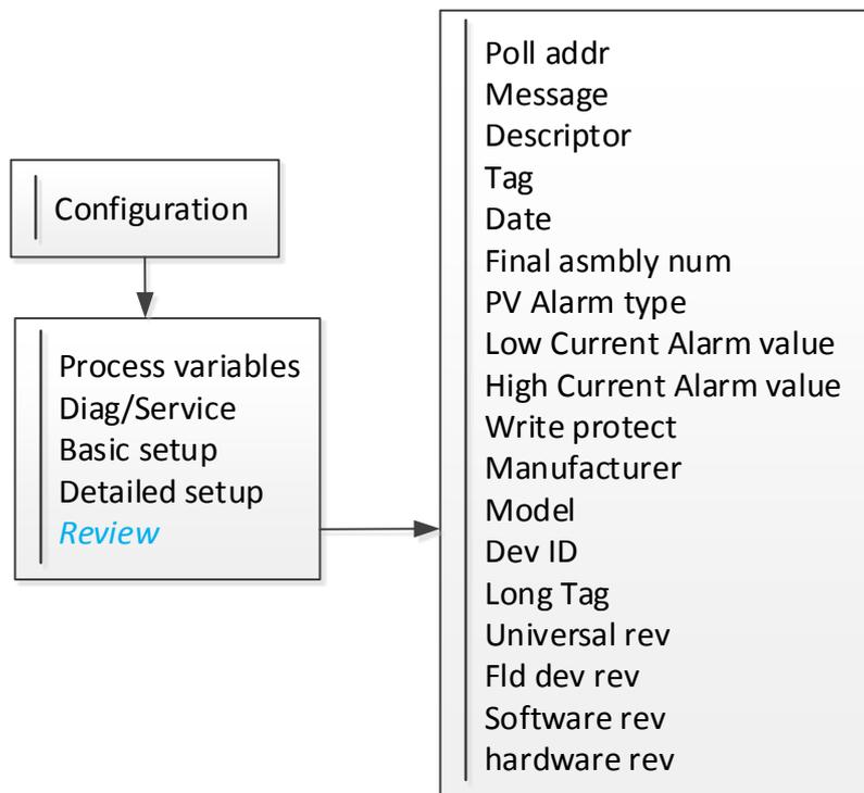
Figure A-5 : NCS-TT106H-R Field Communicator Menu Tree - Detailed Configuration
