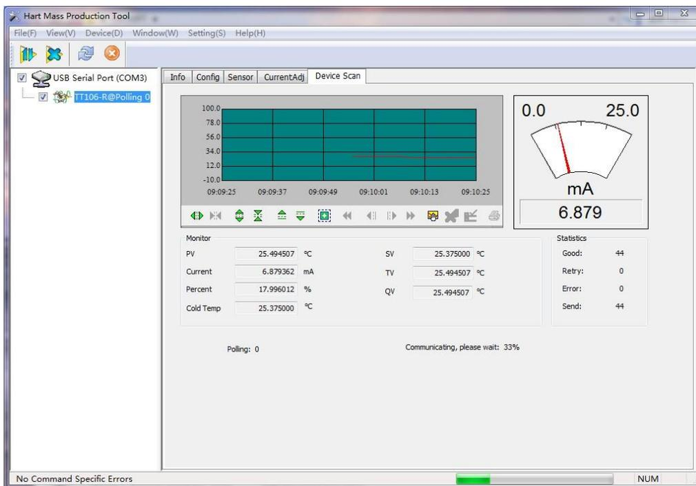
Periodically refresh the dynamic variables of the selected equipment and display the trend curve of the primary variable of the current equipment.
