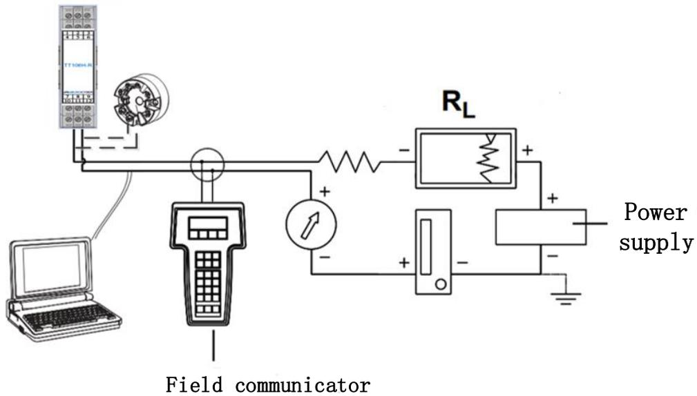
**Note :** The signal loop can be grounded at any point or not grounded.◦
