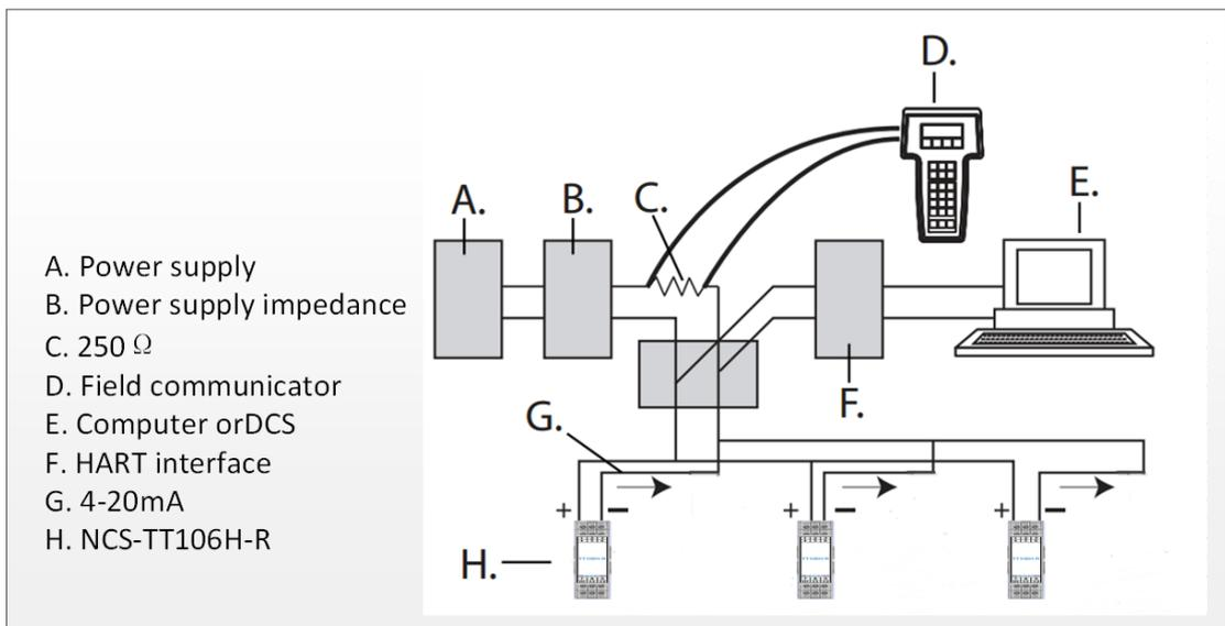
**Note :** The polling address of the NCS-TT106H-R transmitter is set to 0 at the factory, which allows operation with a 4-20 mA output signal in a standard point-to-point manner. If you wish to activate multipoint communication, the transmitter polling address must be changed to a number in the range 1-63. This change disables the 4-20mA analog output, making the output 4mA. The fault mode current is also disabled at this time.
