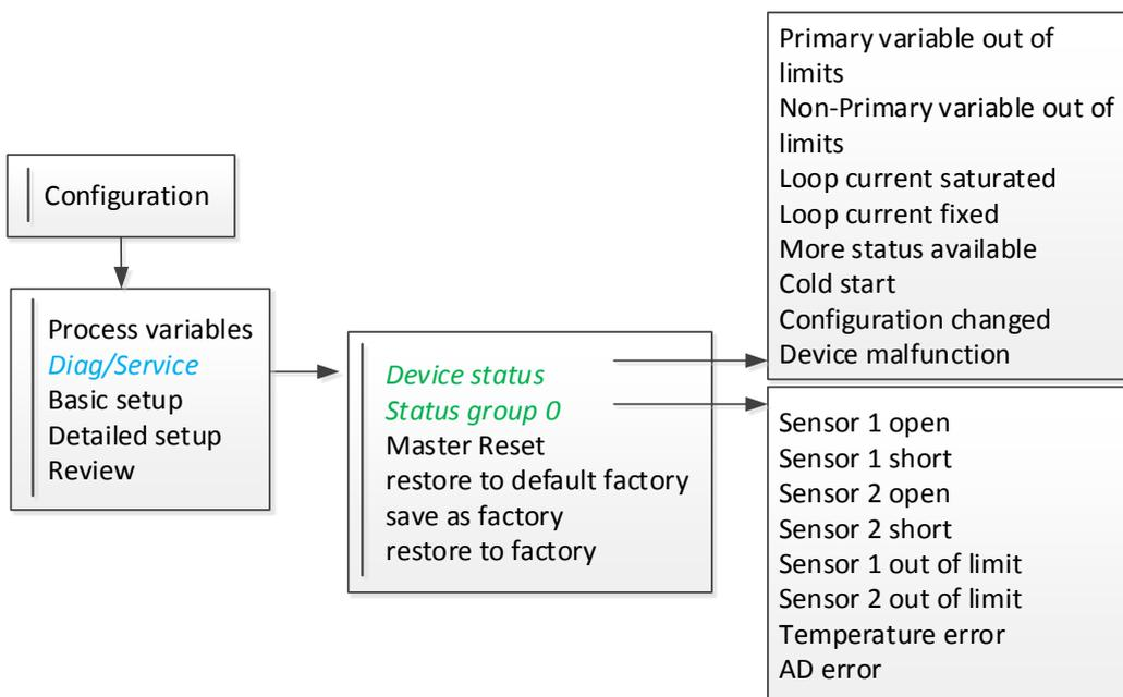
Figure A-3 : NCS-TT106H-R Field Communicator Menu Tree - Basic Configuration
