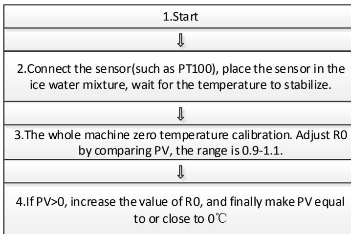
R0 adjustment factor is the zero temperature calibration of the whole machine (transmitter + sensor)
